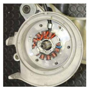
Install the 2 flywheel cable outlet plates (Fig.2 - 12).
