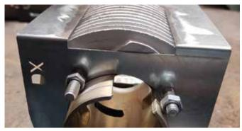
Use the grinding disc to mill (Fig.2 - 1) the side of the cylinder making full length passes, reaching up to the base of the template.
