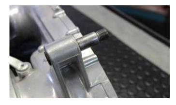
Use the grinding disc (Fig.2 - 1) grind the edge of the pin to allow proper ejection of the pin.
