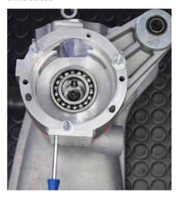
Insert the seeger present in the set (Fig.2 - 10) in the groove of the Chimera block.
