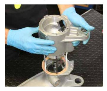
Screw the nuts and washers onto the M6X190 threaded rods previously installed in positions «B» «D» «F», the M6 nuts and relative large washers present in the set (Fig.2 - 6). Tighten the nuts to bring it into position definitive conversion Chimera.
