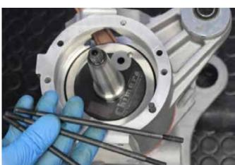
Install the M6x25 dowel present in the grain screw kit (Fig.2 - 5) in position «F». The part of the grain that comes out must have a height of 13 mm.
