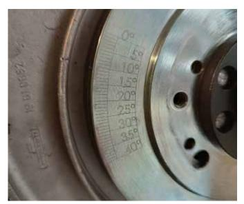
Take a barrel as a reference and position the piston at top dead centre.
