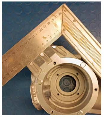
Cutout «3» of the motor limit switch is optional and avoids to interfere with a small portion of the fender rear. Alternately it will be enough to bend lightly the rear fender next to motor limit switch.
