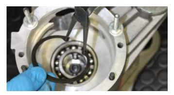
Lubricate the internal seat of the roller bearing and its diameter on the cranckshaft (Fig.1 - A2). Loosen the 3 M6 nuts previously screwed on threaded rods to allow the 2 shafts to define the their natural position during their tightening. Heating and insert inner roller bearing "B" on crank until the specific shoulder diameter.
