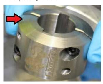
Position the collar in order to allows you to insert the keys. With the Allen key, inserted into one screw of the collar, hold it in place. Insert the keys in their seats up to the stop (present on the tree).
