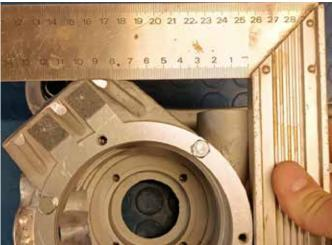
The cut <2> must be parallel (2 // 4) to the template cutting edge and with an offset of 3.00 mm from the end of the template and perpendicular to the plane of the support that is being cut.
