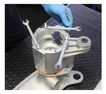
Set, without tightening, the M8X30 screws and washers e M6X35 of the set (Fig.2 - 5) in the same positions views for checking the chimera and casing assembly engine (see PHASE 2).
