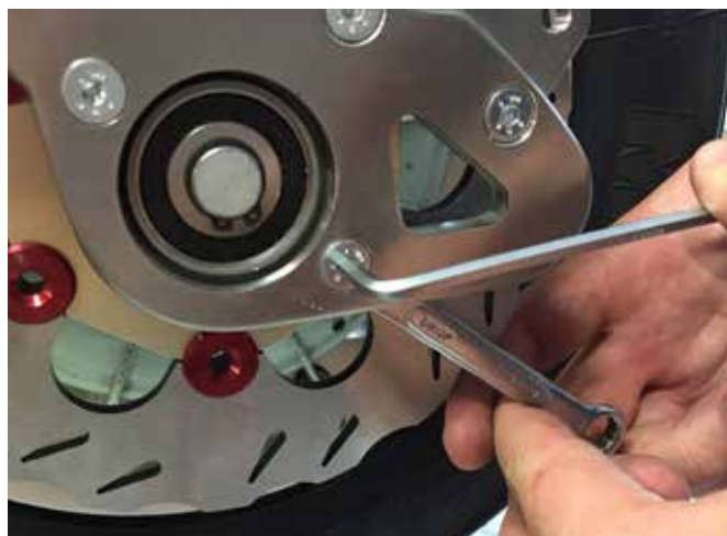
05 Temporary fit the clamp ( pic. 1 - N ).
