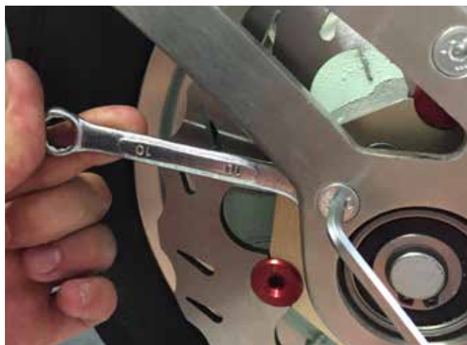
04 Screw and secure the bearing assembly.
