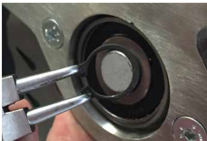
03 Put retainer seeger on disk support pin.
