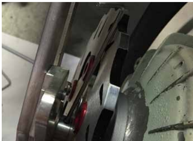
03 Put retainer seeger on disk support pin.
